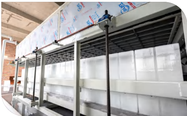
Commissioning site of 10t automatic ice block ice machine
